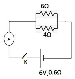
Calculate resistance of the circuit when the key K is:
